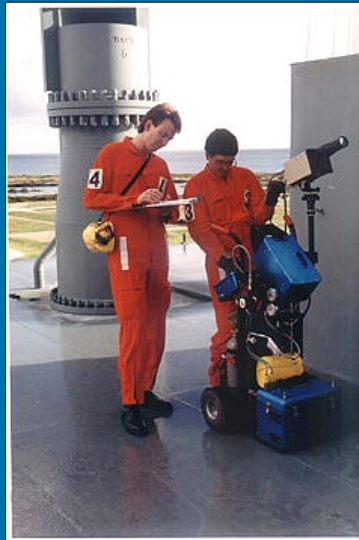
Ice Team performs inspection of ET after tanking
